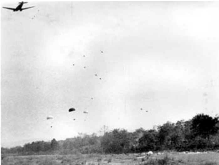
Planes from the 2 nd Troop Carrier Squadron drop supplies to the 5307th. Supply drops were always from altitudes of less than 300 feet. The plane shown here is a C-47 at 200 feet. It is free dropping 100-pound sacks of mule feed and grain, which are dropping faster than the parachuted supplies dropped by the preceding plane. Feb 1944; From http://www.marauder.org/
